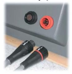
POWER <u>OUTPUT</u> FROM THE PROVIDED NAUTICOMP POWER SUPPLY IS TO BE 12.4VDC. PLEASE DOUBLE CHECK BEFORE CONNECTING TO THE DISPLAY FOR THE FIRST TIME.
