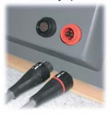
POWER OUTPUT FROM THE PROVIDED NAUTICOMP POWER SUPPLY IS TO BE 12.4VDC. PLEASE DOUBLE CHECK BEFORE CONNECTING TO THE DISPLAY FOR THE FIRST TIME.
